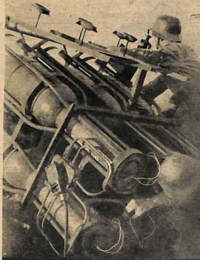
This photograph released by the Germans, shows a gunner adjusting the firing leads to a rocket-launching apparatus.
