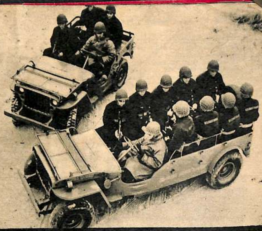
Here is the jeep's big brother, a new Coast Guard version which is only three feet longer than the original, but carries nine men and a driver. The new jeep gallops along beaches at 60 miles per hour.
