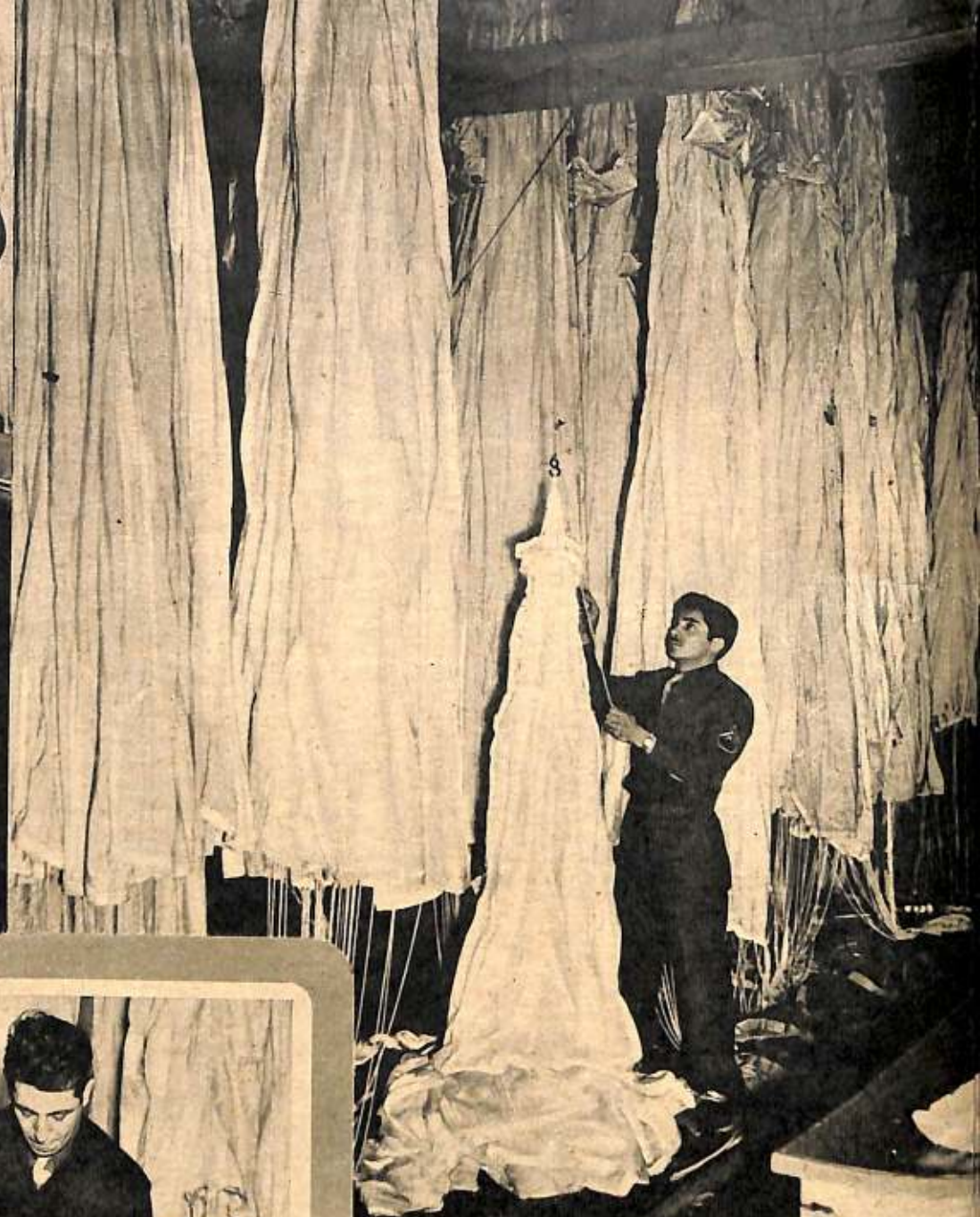
Inspected, they are hung in a heated room for twenty-four hours and must be completely dry before removal.
