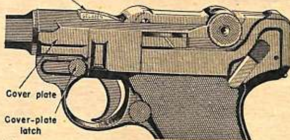
Close-up of Luger pistol to show operation of extractor.
