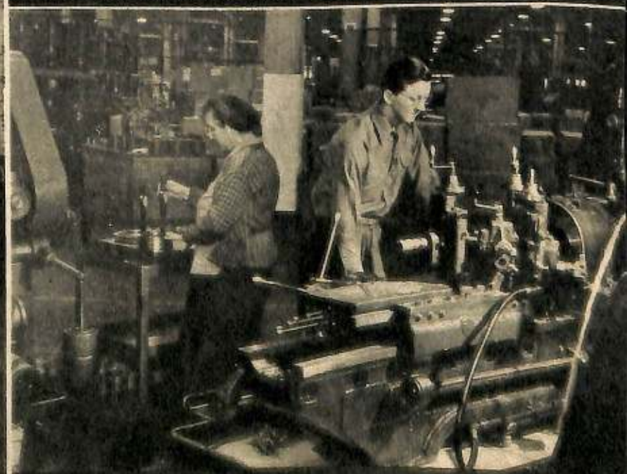
Legs working at his turret lathe in the Dodge plant. His machine cuts sleeves for the oil system of B-29 engine propeller shafts.
