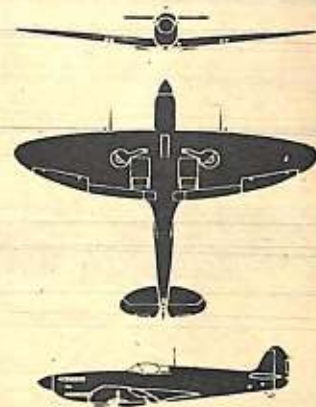
SPITFIRE. Because of its elliptical wing the British Spitfire might be mistaken for Japan's "Val"—but only at a split-second view, since the Spit has retractable landing gear. Otherwise it has features of a United Nations fighter. Look for spinner on pointed nose and for the radiator intakes under wings.
