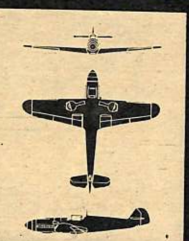
ME-109. The German Messerschmitt fighter looks like a flying torpedo, because of the thick nose with an even taper to its in-line engine. One feature gives it away, even at a distance: the stabilizer set high on the fin and rudder. The wing tips of the ME-109 are rounded and the wings' trailing edges taper.
