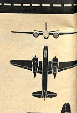
"HAMP." Another Mitsubishi product which, in fact, is a sort of M-2 Zero. For recognition purposes, the only significant difference between the two planes is the squared wing tips of the Hamp. At an angle this Japanese plane might be confused with the U. S. Wildcat because of its squared wing tips.
