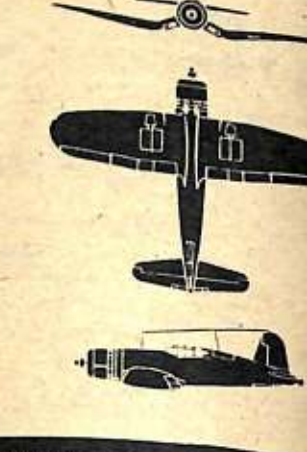
F4U CORSAIR. Along with the Stuka and the P-38 the Corsair is one of the most easily recognizable of all military airplanes. It gets that way by its inverted gull-wing design. It has a long nose fronted by a radial engine; the pilot sits almost amidships. Rudder is set forward on rounded fuselage.
