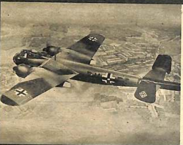
DO-217. Introduced about two years ago, this Dornier heavy bomber packs a mean punch. Like the JU-88 it has quite a lot of nose and quite a few guns in it. As you see, the fuselage is long and thin with twin fins and rudder. Long distance from wing to tail gives the DO-217 a stretched-out appearance.
