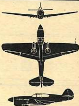
P-40 WARHAWK. This familiar war horse is a ruler-straight job with a long nose and a deep radiator, its most distinguishing feature. It has a big spinner fairing into the fuselage in front of the heavy radiator. Note the P-40's heavy straight taper on trailing edges of wings, which have rounded tips.
