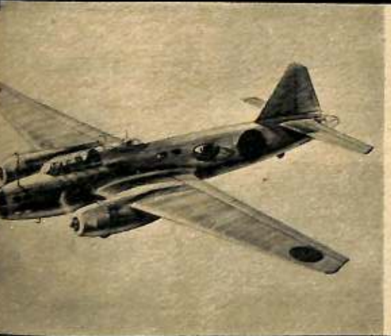
"BETTY." Another Mitsubishi, Type 1, medium bomber. Betty has a very thick body and from the side looks like she might be able to take off in either direction. There is plexiglas aplenty, in nose and tail and in blisters on either side at the waist. There is a turret topside and the tail is large and triangular.
