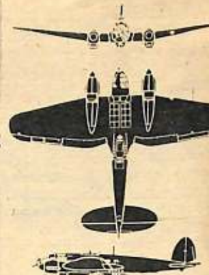
HE-111. The Heinkel medium bomber has one outstanding feature which, if seen from above or below, establishes its identity immediately: the deep "bite" into the trailing edge of the wings as they join the fuselage. From the side it reveals an unusually-designed belly turret aft of the wings.
