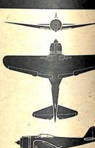
"OSCAR." Still the familiar-type Jap fighter, Oscar has been around almost as long as Zeke. One of its most distinguishing points is the fuselage, which tapers to a very slender appearance at the joining of the tail assembly. The high cockpit cowling allows all-around visibility. There is a full dihedral.
