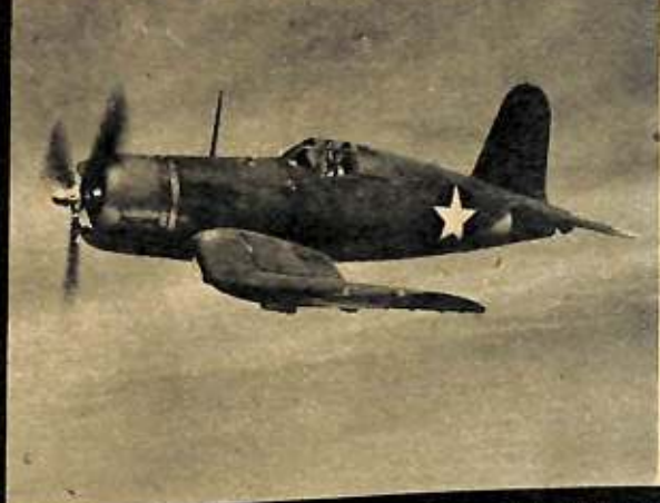
F4U CORSAIR. Along with the Stuka and the P-38 the Corsair is one of the most easily recognizable of all military airplanes. It gets that way by its inverted gull-wing design. It has a long nose fronted by a radial engine; the pilot sits almost amidships. Rudder is set forward on rounded fuselage.
