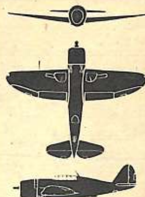
P-47 THUNDERBOLT. For a fighter the Thunderbolt is a fat ship (compare figure of the pilot here with pilot in Warhawk). The shape of its wings remotely suggests a Spitfire or a Jap "Val" dive bomber but other features—radial engine, fat belly and sharply tapered tail—easily distinguish it as ours.
