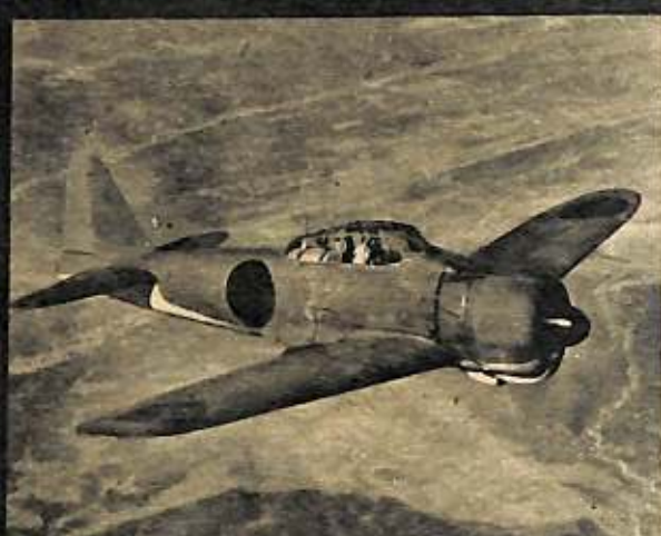
"ZEKE." Mitsubishi's famous Jap fighter—the Zero—is a much praised and often-shot-down airplane, which looks less like any Allied plane than other Nip ships. It might be confused with the U. S. Navy SBD (Dauntless) but is slimmer and does not have our own ship's graceful curves at wing roots and tail.
