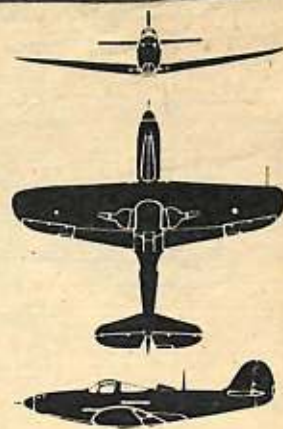
P-39 AIRACOBRA. This is the baby with the turned-up nose, and by the pert flip of her tail and nose she's recognizable. In fighters there is nothing quite like her, although either a P-40 or an ME-109 might appear similar. The rocking-chair effect and the long nose and center-set wings identify her.
