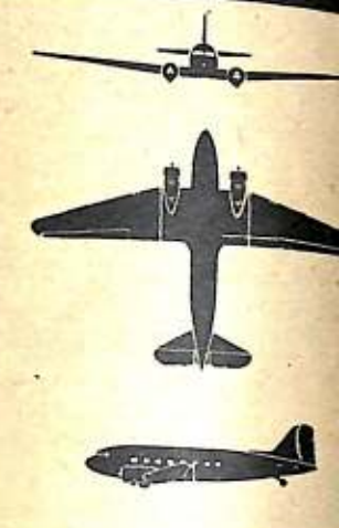
C-47 SKYTRAIN. This old baby is the familiar commercial air liner seen every day in the States for several years past. In flight it can't quite tuck its wheels all the way up. Leading edge of the wings taper sharply. Center wing section of a C-47 has no dihedral but the out-panels slope up gracefully.
