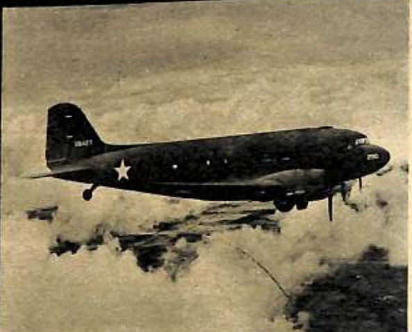
C-47 SKYTRAIN. This old baby is the familiar commercial air liner seen every day in the States for several years past. In flight it can't quite tuck its wheels all the way up. Leading edge of the wings taper sharply. Center wing section of a C-47 has no dihedral but the out-panels slope up gracefully.
