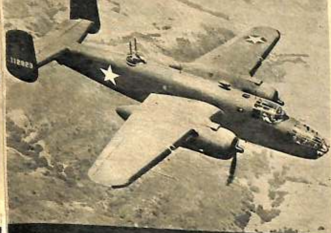
B-25 MITCHELL. This medium bomber has an unusually long nose, giving the impression that there's more of it in front than behind the wings. From below watch for similarity between Mitchell and Dornier 217. The B-25 has a slight gull wing appearance because of the dihedral of inboard panels only.
