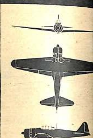
"ZEKE." Mitsubishi's famous Jap fighter—the Zero—is a much praised and often-shot-down airplane, which looks less like any Allied plane than other Nip ships. It might be confused with the U. S. Navy SBD (Dauntless) but is slimmer and does not have our own ship's graceful curves at wing roots and tail.
