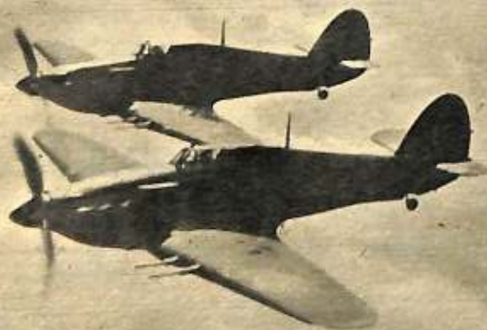
HURRICANE. This versatile British aircraft resembles no German plane. It has a hump-backed fuselage and a very pointed nose, with a small and sharp spinner. There is a large air scoop below the cockpit on the underside and a large fin and rudder with a cut-in on the trailing edge of the elevator.
