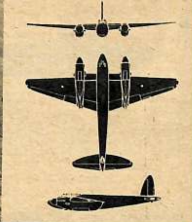
MOSQUITO. The British light bomber-fighter is a sleek job with several easily recognizable features: underslung in-line engines, which protrude nearly as far forward as the nose; high, upright tail; slim fuselage with the wings wide at the base and then tapering out into sharp rounded tips.
