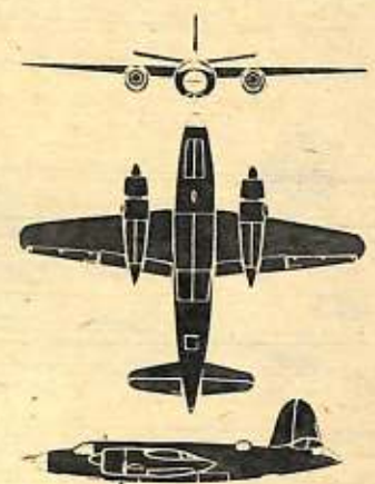
B-26 MARAUDER. Like "Betty" the Marauder has a lot of body at both ends. Like the Jap bomber its fuselage is cigar-shaped. Differences can be noticed most quickly in the tail assembly. Single fin and rudder of B-26 is tall. Tail plane sits high and engine nacelles protrude aft of wing.
