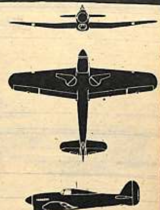
TYPHOON. The deep scoop of this British high-altitude fighter sets it apart, making it resemble a gasping fish. Seen head-on the dihedral (the upward sloping of the wings) is on the outer panels only. Fin and rudder are extended slightly below the fuselage. Wings and tail plane are similar in shape.
