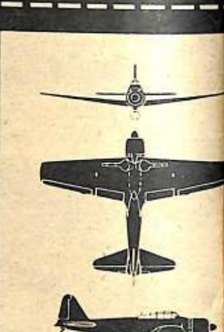
"HAMP." Another Mitsubishi product which, in fact, is a sort of M-2 Zero. For recognition purposes, the only significant difference between the two planes is the squared wing tips of the Hamp. At an angle this Japanese plane might be confused with the U. S. Wildcat because of its squared wing tips.
