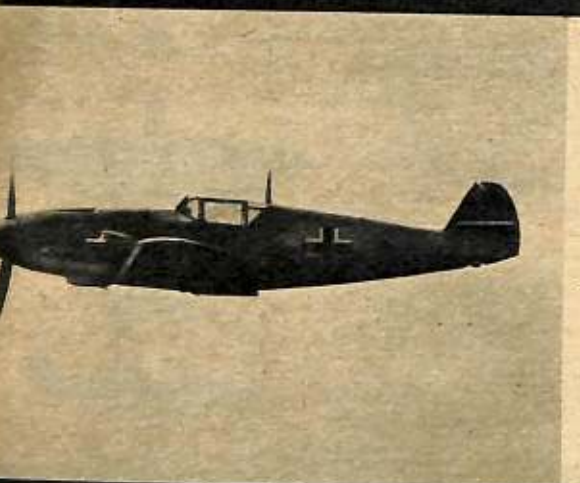
ME-109. The German Messerschmitt fighter looks like a flying torpedo, because of the thick nose with an even taper to its in-line engine. One feature gives it away, even at a distance: the stabilizer set high on the fin and rudder. The wing tips of the ME-109 are rounded and the wings' trailing edges taper.
