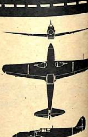
"TONY." This is one of the newest and hottest of Jap fighter planes and it is a radical departure from anything previously dished out by Japan. Tony is an inline-engined job, unique in Nip fighters, and from an angle it might carelessly be mistaken for either a U. S. Mustang or a P-51 Mustang.
