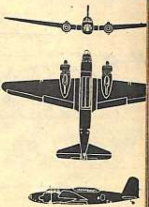
"SALLY." The Mitsubishi 97 medium bomber, which does a great deal of work for Tojo. Sally could hardly be confused with any other two-engine plane of any nation, principally because of the long cockpit enclosure, which is in two sections. The rear greenhouse characteristically juts above the fuselage.
