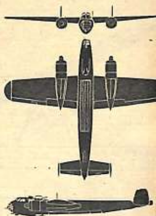
DO-217. Introduced about two years ago, this Dornier heavy bomber packs a mean punch. Like the JU-88 it has quite a lot of nose and quite a few guns in it. As you see, the fuselage is long and thin with twin fins and rudder. Long distance from wing to tail gives the DO-217 a stretched-out appearance.
