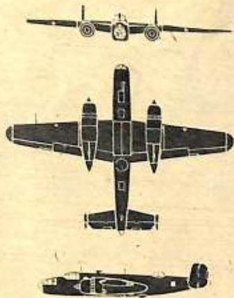
B-25 MITCHELL. This medium bomber has an unusually long nose, giving the impression that there's more of it in front than behind the wings. From below watch for similarity between Mitchell and Dornier 217. The B-25 has a slight gull wing appearance because of the dihedral of inboard panels only.
