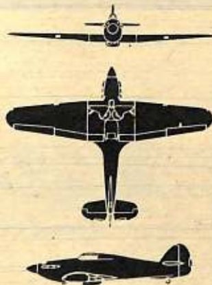
HURRICANE. This versatile British aircraft resembles no German plane. It has a hump-backed fuselage and a very pointed nose, with a small and sharp spinner. There is a large air scoop below the cockpit on the underside and a large fin and rudder with a cut-in on the trailing edge of the elevator.
