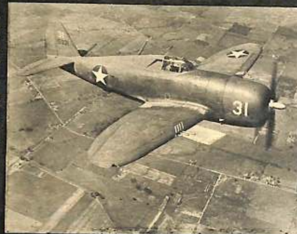
P-47 THUNDERBOLT. For a fighter the Thunderbolt is a fat ship (compare figure of the pilot here with pilot in Warhawk). The shape of its wings remotely suggests a Spitfire or a Jap "Val" dive bomber but other features—radial engine, fat belly and sharply tapered tail—easily distinguish it as ours.
