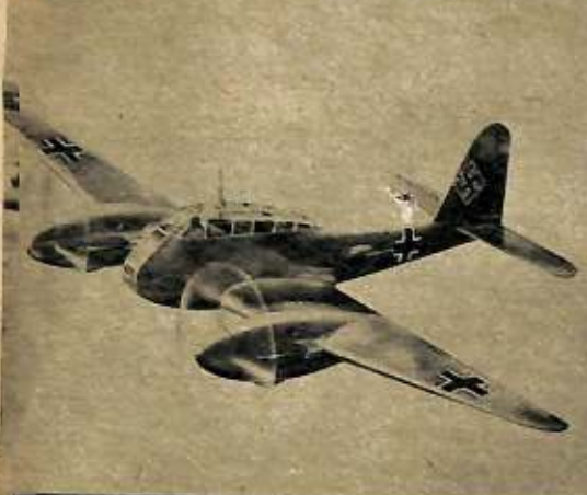
ME-210. This fighter-bomber can be spotted by many unusual features. The tail seems out of all proportion with the thin fuselage on one end, while the nose gives way to a great bulged greenhouse at the other end. Guns at the waist are remotely controlled and fire from blisters on the sides of the fuselage.
