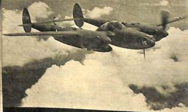
P-38 LIGHTNING. Because of the twin tail booms, it's practically impossible to confuse the Lightning with any other ship. However, Germany has three types of aircraft with twin booms: one a float plane, one a glider and one a recon ship (FW-189). The FW-189 is bigger, slower, more bulky than the P-38.
