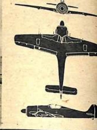
FW-190. This is the only German single-engine fighter with a radial engine. Because both the Focke-Wulf job and our P-47 have radials, they may be confused. In head-on view FW-190 has fuselage on top of wing, while P-47's belly bulges below wing. Tails also differ, FW-190's being thin and square.
