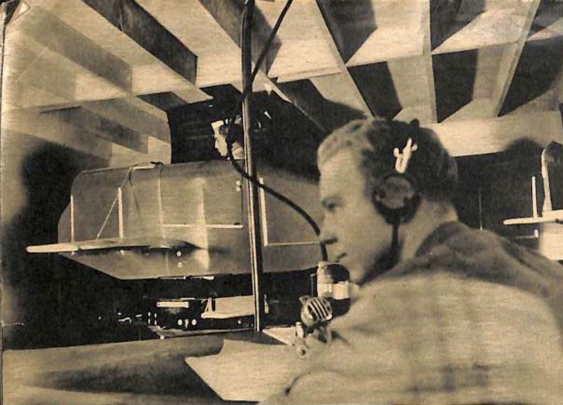
EARTHBOUND. The Link Trainer, used in ground training of glider cadets, is invaluable to both instructor and student, duplicating all the maneuvers of the plane.
