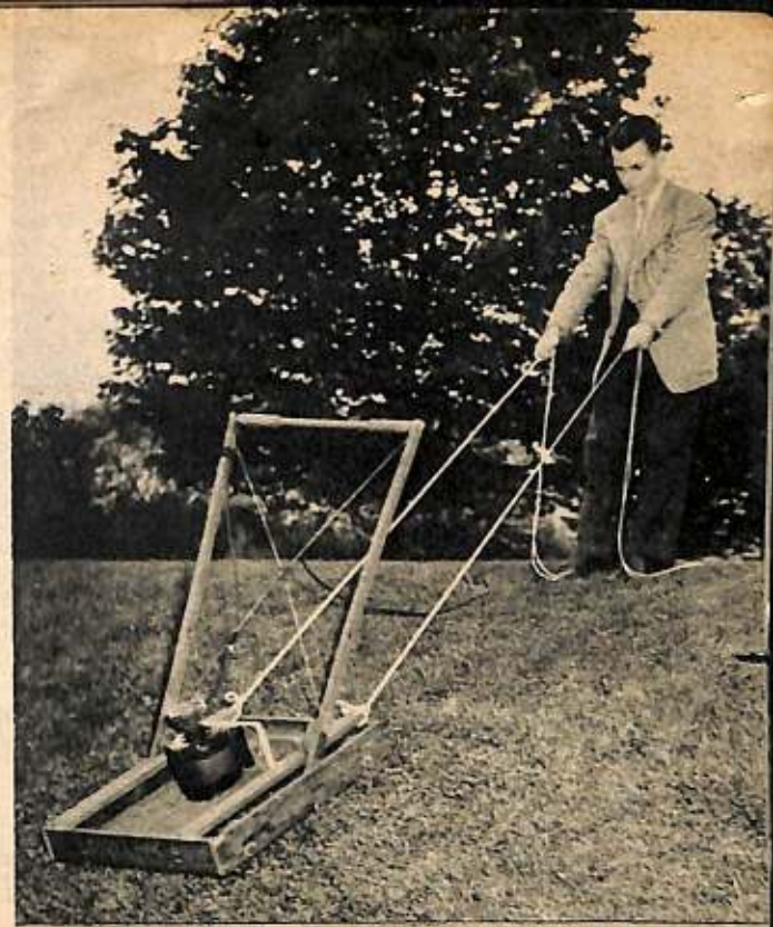
LAWN MOWER. JIM TUSKA, OF PHILADELPHIA, IS SHOWING OFF HIS DAD'S GRASS-CUTTER MADE FROM OLD RAZOR BLADES AND A VACUUM CLEANER.
