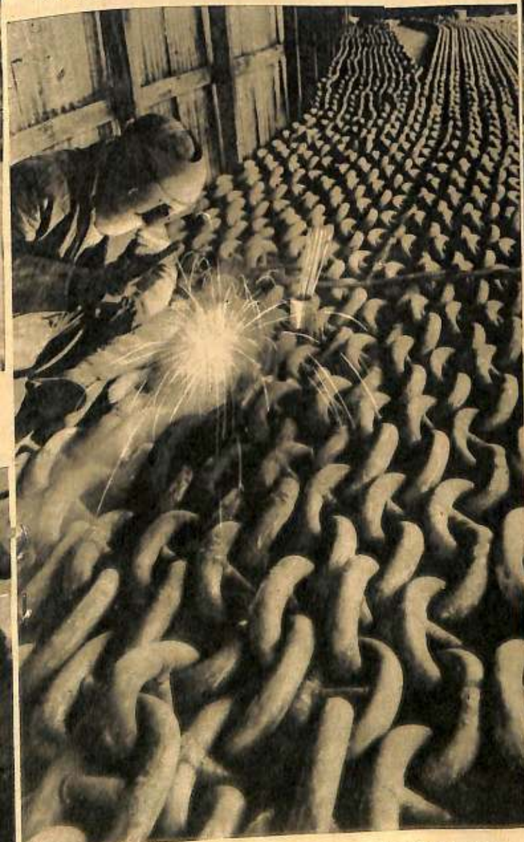
CLANK, CLANK. A few dainty, 50,000-pound strands of chain which a Vancouver factory is turning out for Liberty Ships. No stronger than their weakest links, perhaps, but still plenty strong.
