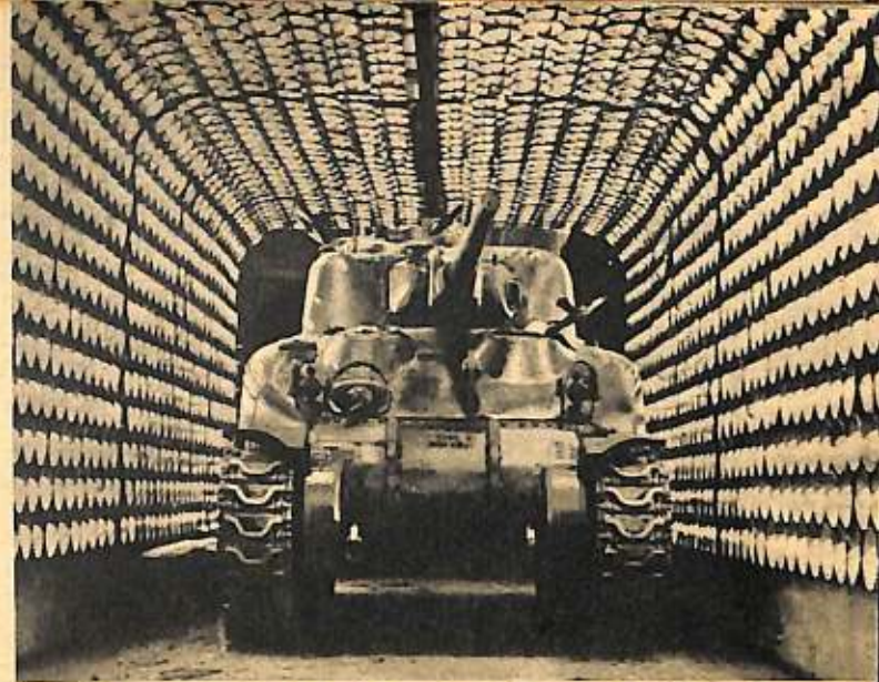
A tank getting a sun-bath in the Army's new infra-red room where a new paint job dries in four minutes.
