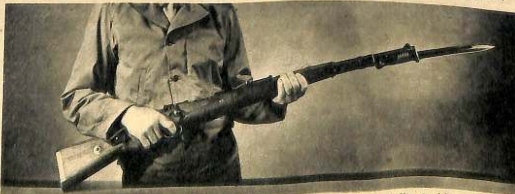
German Model 98K, a short bolt-action Mauser, fires a 7.92-mm bullet (caliber .31).
