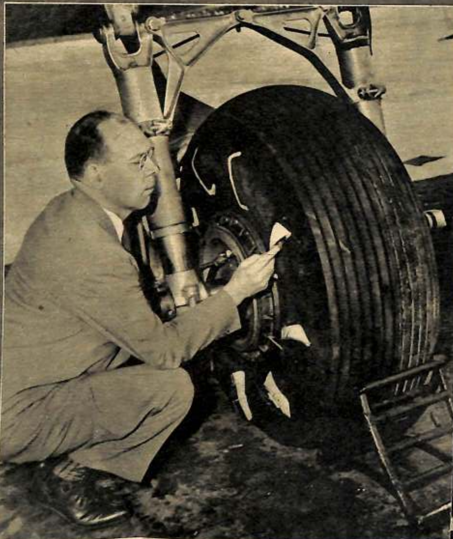
A new invention designed to double, almost, the life of plane tires. Those rubber fins, outlined in white on the sidewall, open when the plane's landing gear is lowered, catching the wind and starting the wheel spinning.
