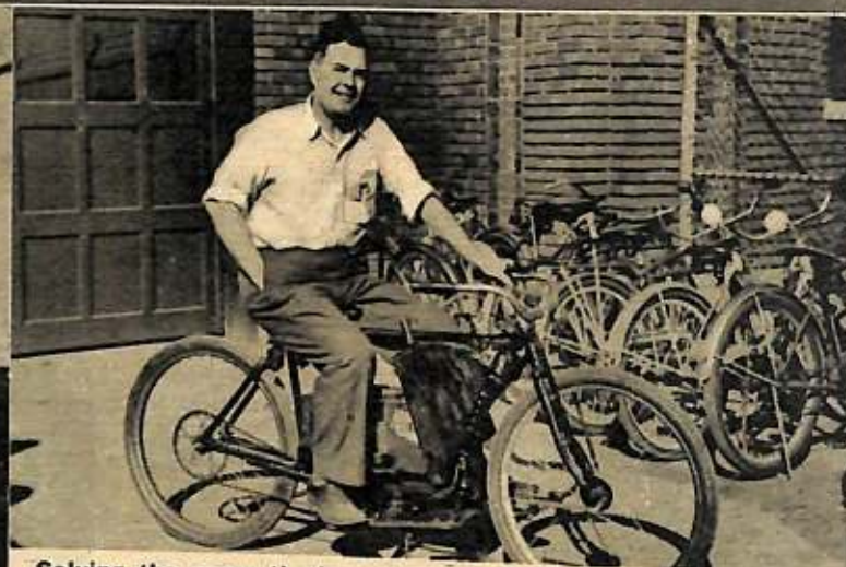
Solving the gas-rationing problem, this war worker in South Bend, Ind., has rigged his bike up to run on a couple of three-cell automobile batteries.
