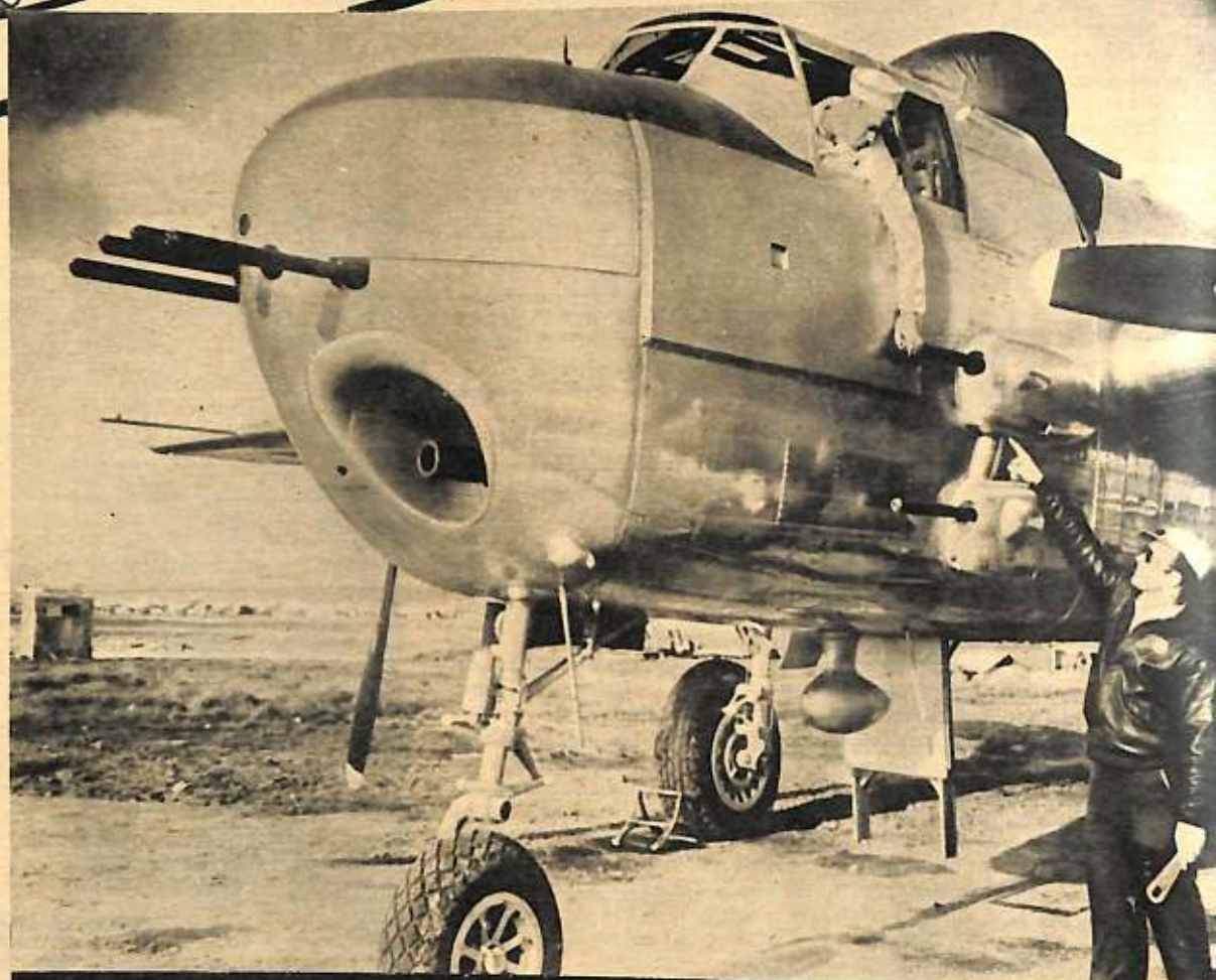
BACKING UP THE BOMBS. The B-25 Mitchell now totes nearly five times the armament of those which bombed Tokyo. Eight more guns you can't see: Two on the other side of the pilot's compartment, two in the waist, two in the upper turret, and two in the tail.
