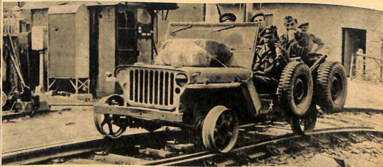
RAIL JEEP. Just to prove it can do anything, this jeep sets out to provide some competition for the railroads. Special wheels replacing the usual tires enable it to hoot up and down these tracks in France.
