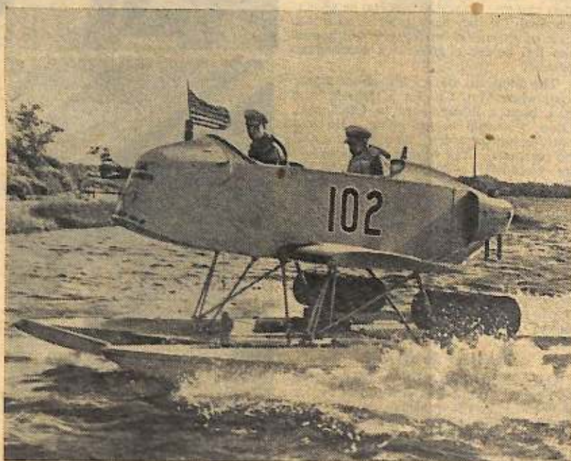
A new U.S. vessel, designed for anti-submarine patrol, is put through tests on the U.S. East Coast. Powered by an aerial engine, the craft skims along the water's surface at 50 miles an hour, and according to its inventor it cannot be detected by underwater listening devices. The boat is armed with four depth charges, a light cannon and machine-guns and can be hoisted and carried on any vessel as easily as a lifeboat.
