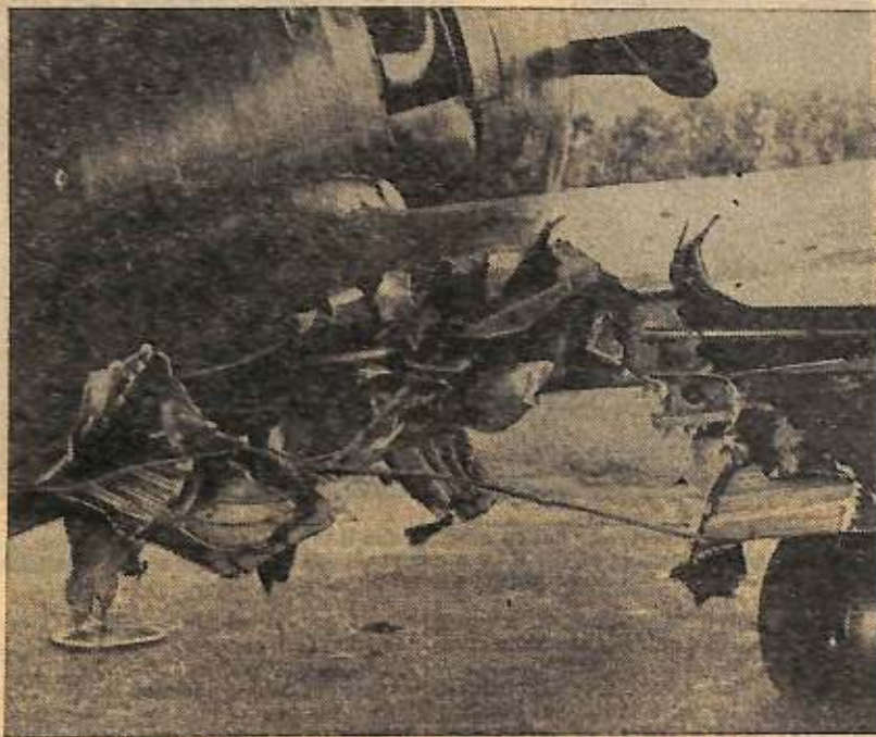
After five 20mm. shells had plowed into the right wing of his P47, Lt. Justus Foster, of Junction City, Kan., recovered his plane from a spin of 10,000 feet, and limped to safety in England with his plane in this condition.
