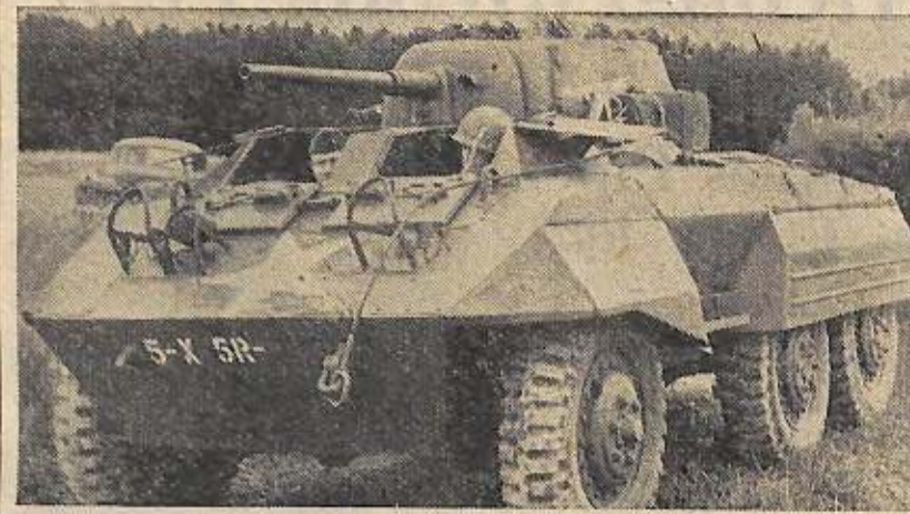
The M8, latest combat vehicle added to the Army's mechanized equipment, was built to combine the speed and maneuverability of an automobile with the punch and armor protection of a light tank. It is a six-wheeled, eight-ton car capable of high speed over virtually any type of terrain. It mounts a 37mm. cannon and a .30 caliber machine gun.
