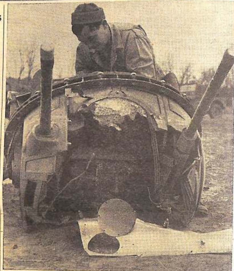
"Stella"—a damaged Flying Fortress—gets a going over (top) by members of a Mobile Repair Unit of the Eighth Air Force at the spot where it was forced to land in England. Cpl. Rodger Case; of Columbus, Ohio (bottom), salvages parts from the Fort's wrecked ball-turret.
