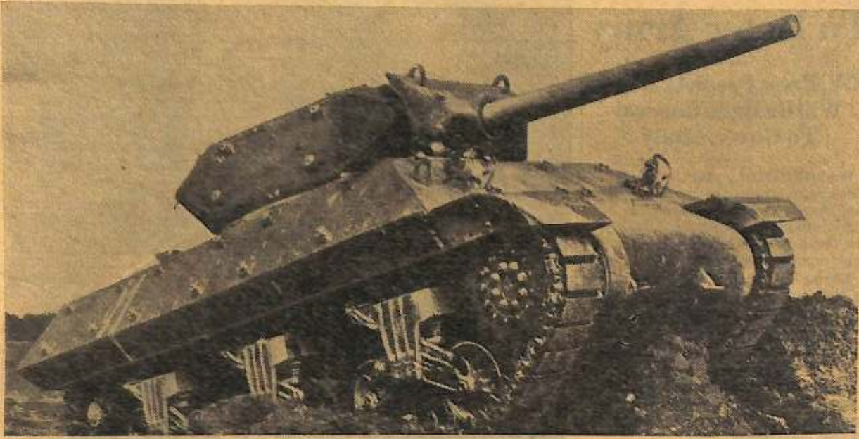
This is a new U.S. tank destroyer whose battle mission is to seek out and demolish enemy armed vehicles. Called the M-10 in Army technical manual, it is heavily armored and faster than the ordinary tank and carries heavy firepower. It already has been tested in battle.
