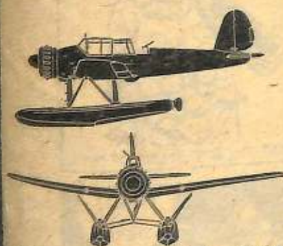
Type: two seat. Speed: 193 max. Ceiling: 23,000 service. Range: 670. Armament: 2 c., 2 m.g. Engine: air-cooled. Length: 38ft. 2 1/2 in. Span: 49ft. 2 1/2 in.
