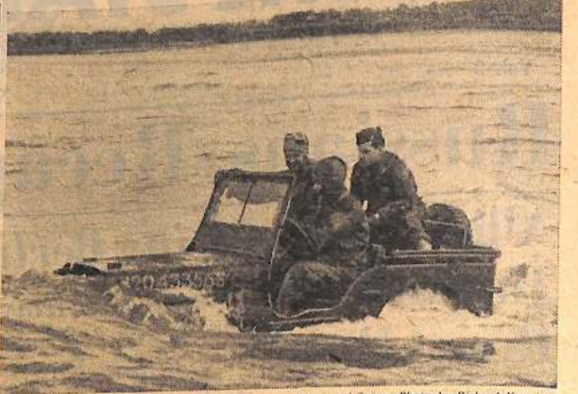
These ordnance men aren't riding in an amphibious jeep, it's just an ordinary one waterproofed by a special process to enable it to ride through water deeper than the top of its radiator.
