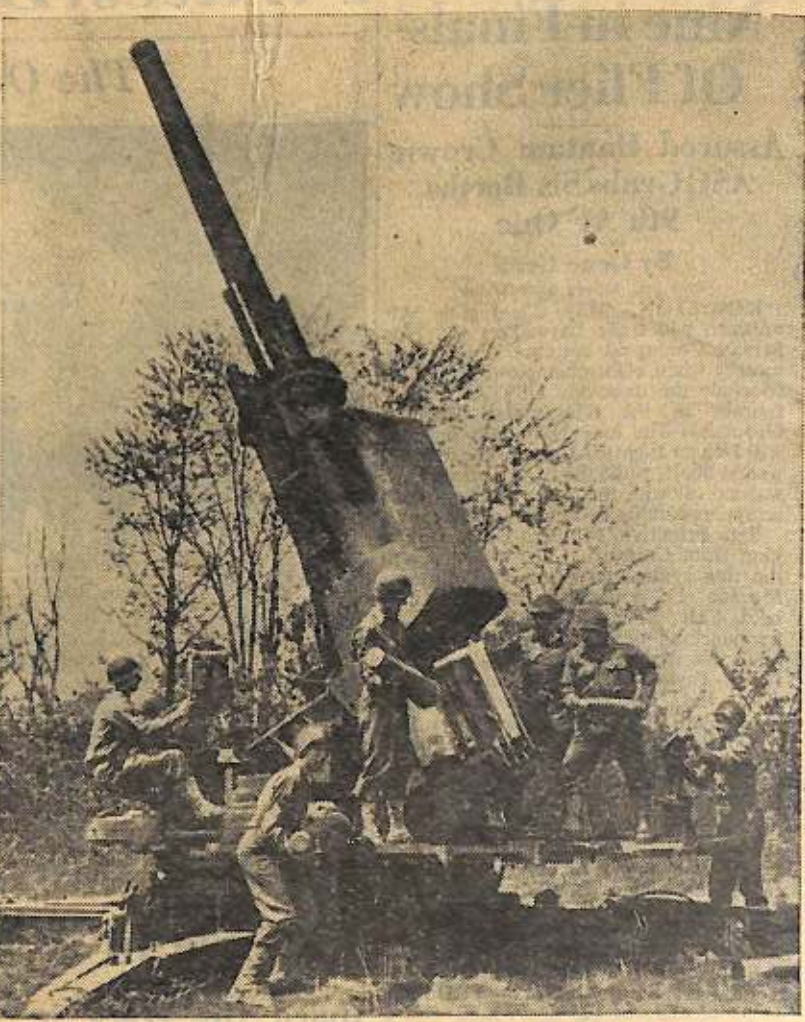
Here's the first picture of the U.S. Army's new "stratosphere gun" which can fire a 120-mm projectile 20,000 feet higher than any other anti-aircraft weapon. The gun, photographed in the U.S., is shown in recoil position with the crew reloading.
