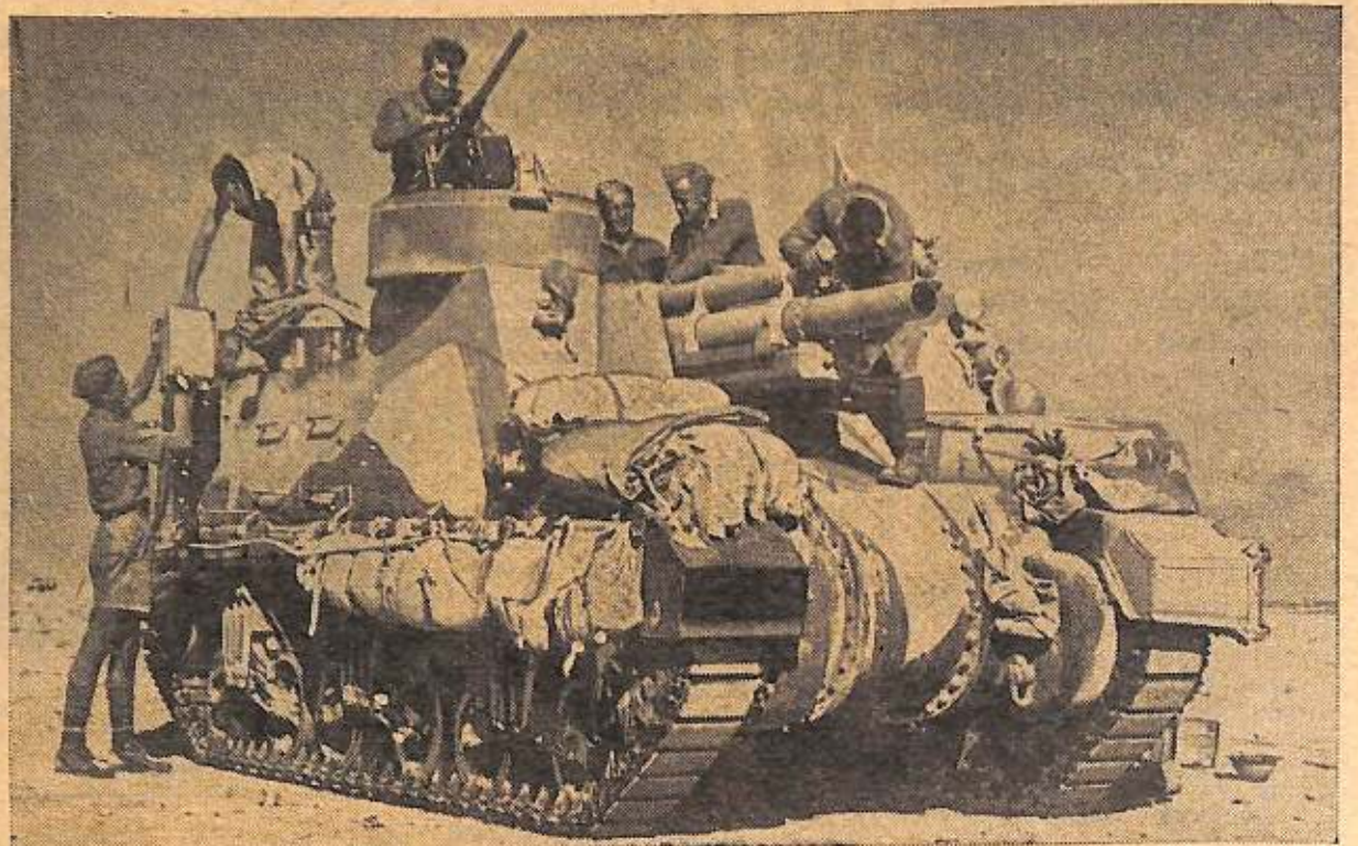
First pictures have just been released of "The Priest"—a 105-mm. self-propelled gun-howitzer which played an important part in Gen. Montgomery's successful rout of the Axis forces now retreating into Tunisia. Known as the M-5 by the U.S. the gun is mounted on an M-3 General Grant tank chassis along with an anti-aircraft gun.
