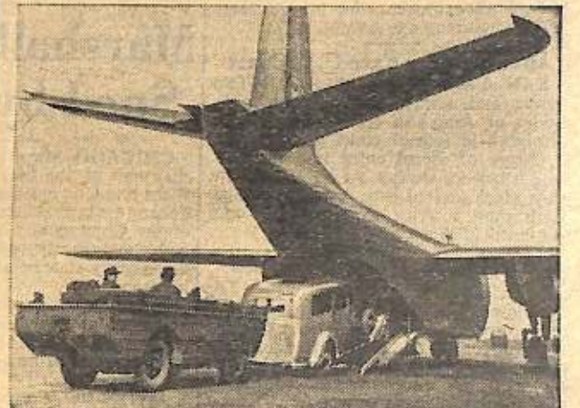
Associated Press Photo The Conestoga, the first U.S. transport plane built of stainless steel, soon will be hauling freight carriage between Fleet bases. A jeep and ambulance go aboard.
