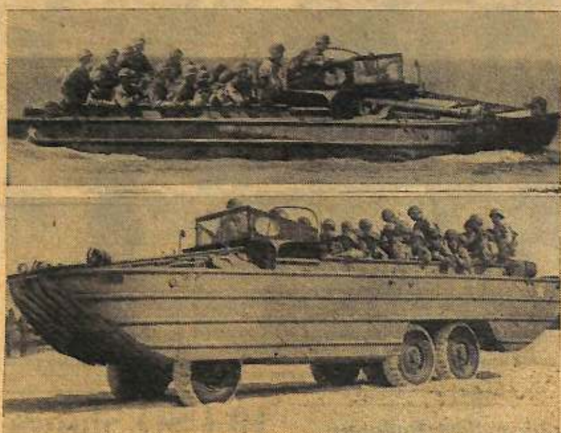
Here's the latest addition to America's invasion amphibious fleet. Nicknamed "the Duck," the two-and-one-half-ton truck is capable of moving 50 fully-equipped troops, weapons or any supplies over water obstacles.
