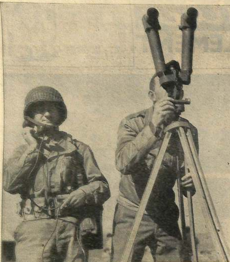
Observers compute data well forward of gun crews who wait for fire orders. T/5 Robert Seitz, of Newville, Pa. (left), relays figures compiled by Capt. James F. McGrath, of DuBois, Pa., with aid of BC scope.
