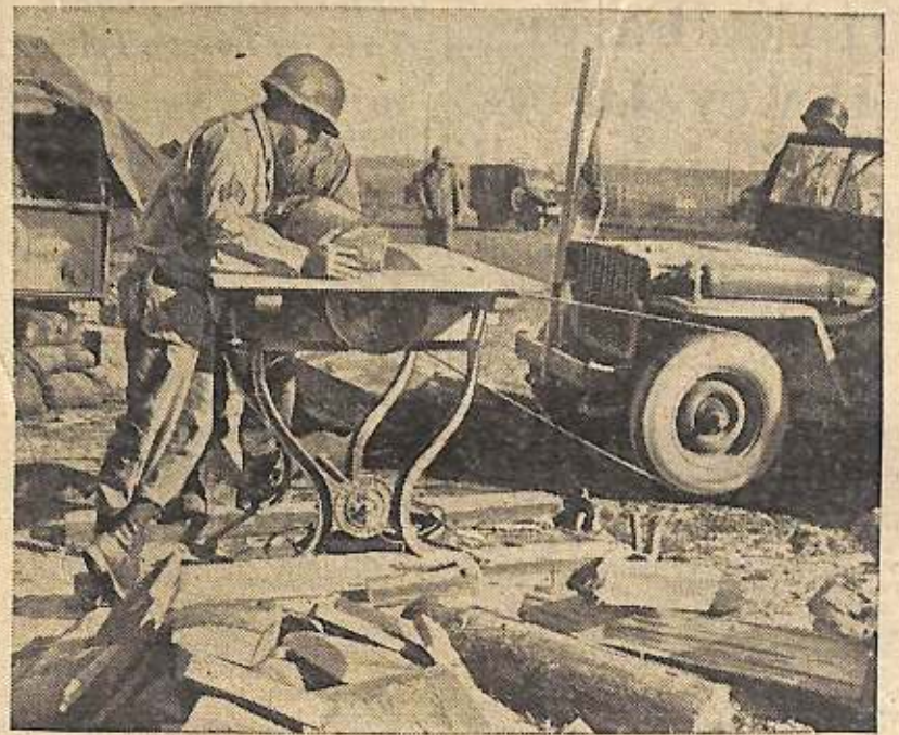
GI Joes serving with the Fifth Army in Italy find a new use for the ever-useful Jeep—serving as powerhouse for a buzz saw.
