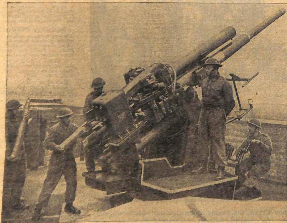
The Crew of a 3.7 inch heavy anti-aircraft gun at a site along England's northeast coast load their piece with a 49-pound round capable of putting up a flak barrage sufficient to blast the Luftwaffe's most heavily armored planes.
